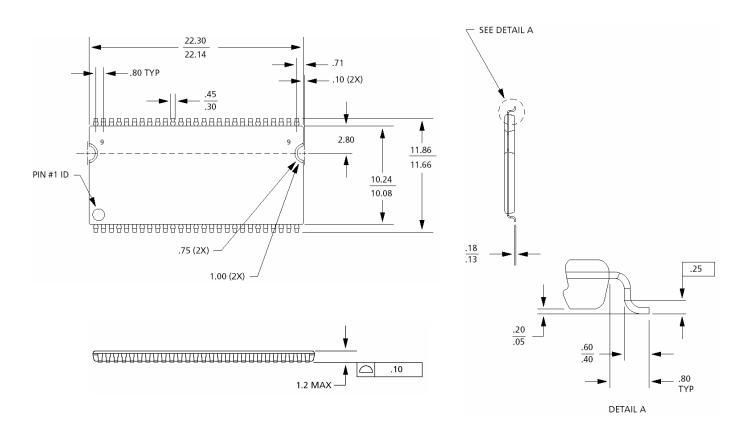
NOTE: 1. All dimensions in millimeters MAX/MIN or typical where noted.
